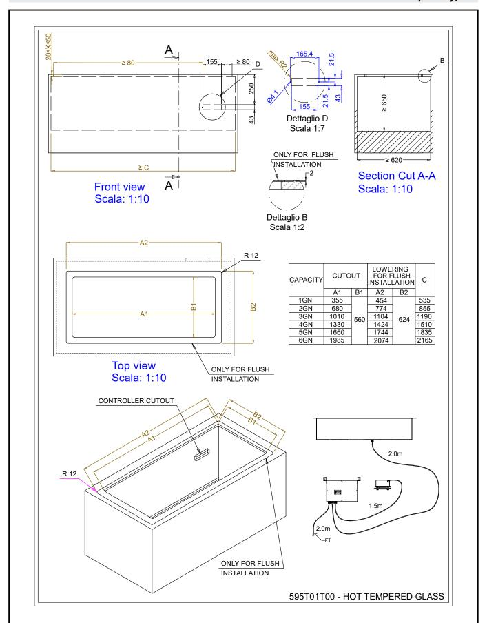
Drop-in tempered glass top (6 GN container capacity)
